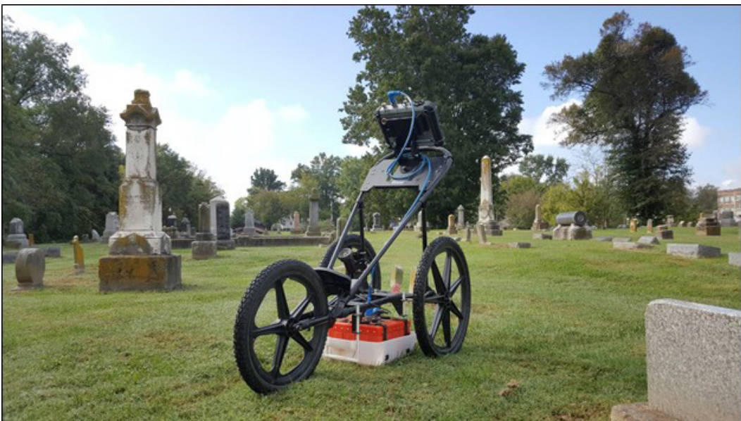
Figure 1. GSSI's SIR ® 4000 control unit and 400 MHz antenna attached to a three-wheel cart.
